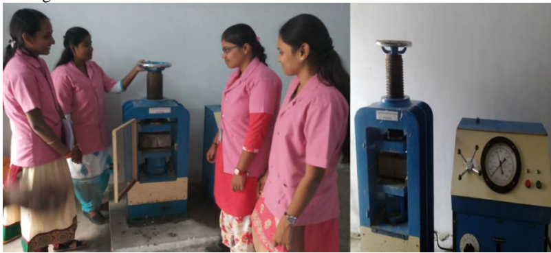
Fig 4.3 Test set up for Flexural Strength Test
