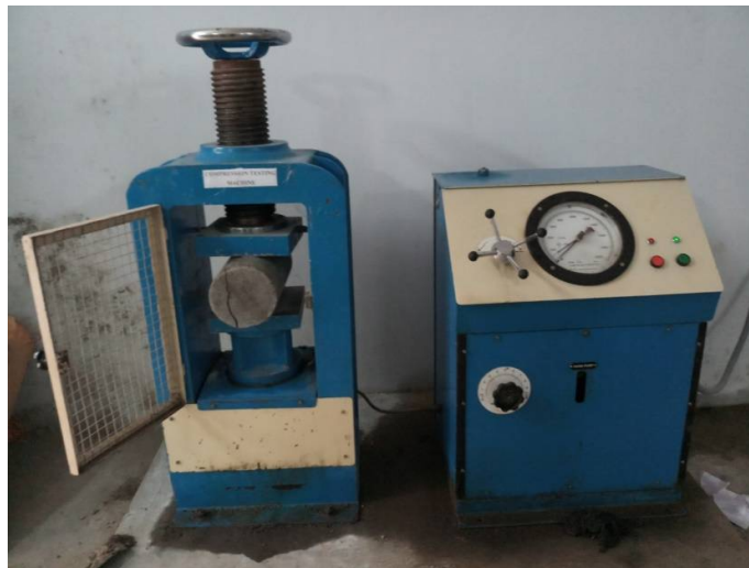
Fig 4.2 Test set up for Split tensile Strength Test
